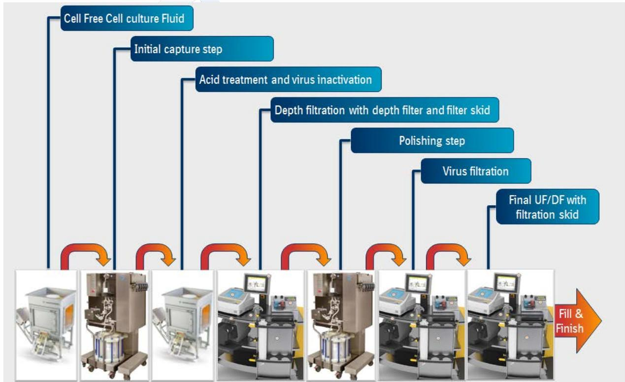
Especially when processing high potent APIs the full disposable upstream and downstream processing reveals its major benefits in a multi-product facility. Hereby the utilized materials are disposed after a processing run or used product dedicated. A change over to the next campaign of a different product is significantly facilitated and safe. 'Cleaning in Place' and 'Sanitation in Place' procedures are not needed and extensive cross contamination analytics can be neglected.
