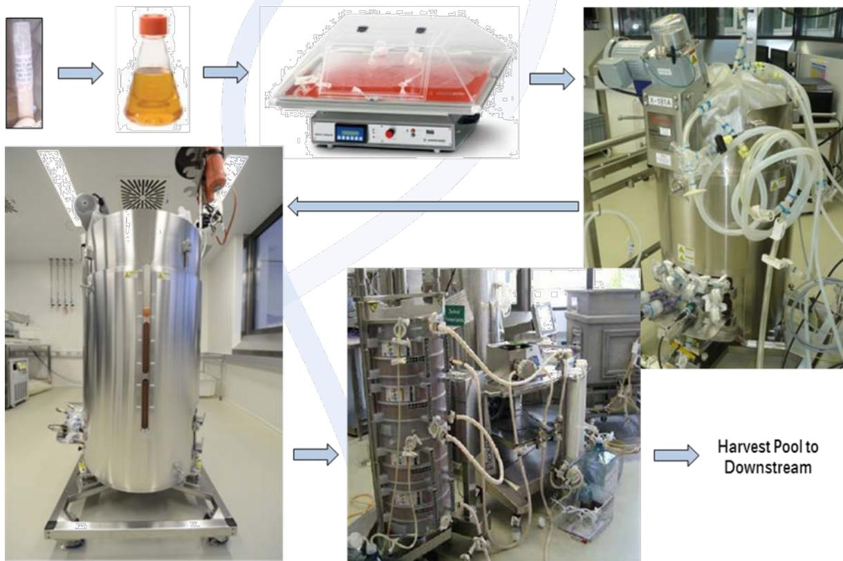
Boehringer Ingelheim is implementing a universal controller system that will enable the use of various single use bioreactor systems (SUBs), such as HyClone, Xcellerex, Sartorius, Millipore, ATMI. Currently, 500 L SUBs from HyClone and Xcellerex have been qualified and used for GMP manufacturing. 100 L and 500 L SUBs will be run as a global platform at Boehringer Ingelheim's sites in Biberach (Germany), Fremont (U.S.A.) and Shanghai (China).
