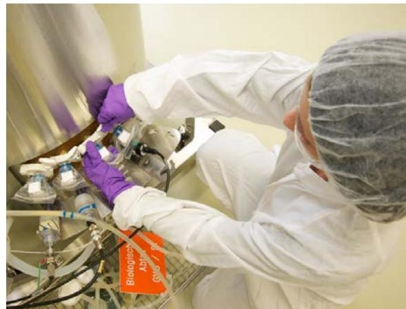
The full disposable upstream process starts in shake flask and bag bioreactor systems on rocking platforms. A standard seed train with 5 passages (15 days in culture) expands the cell culture from
